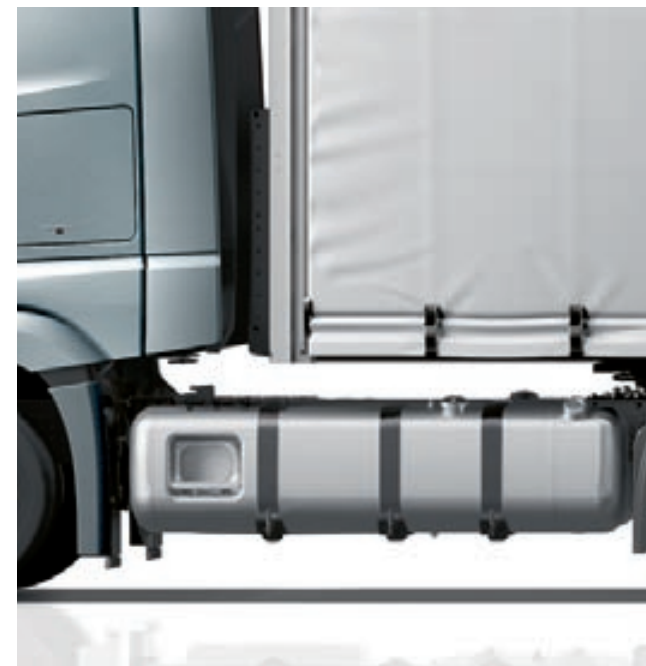
Large volumes and Euro VI as well – with a fuel tank volume of up to 990 l for tractor units and up to 1000 l for low-frame platform trucks, the Actros Volumer provides an especially long range for high-volume haulage.
