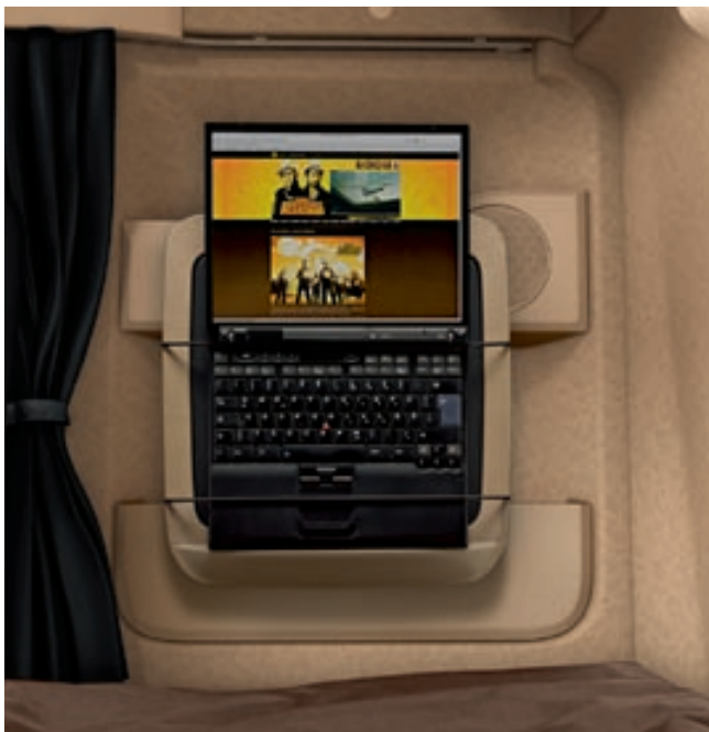
The notebook fixture provides a secure surface for laptops and can be easily stowed away in the open space above the windscreen or in the side panel on the co-driver's side. The laptop can be connected to the Actros's loudspeakers via an Aux-in connection 2) , to give excellent sound when watching a DVD, for example.
