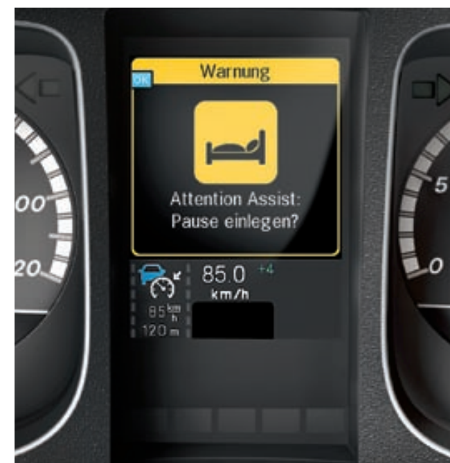
The new Attention Assist 1) system, which is available as an option, can detect signs of increasing tiredness and inattention. It can issue a visual and audible warning sign and recommend the driver takes a break.
