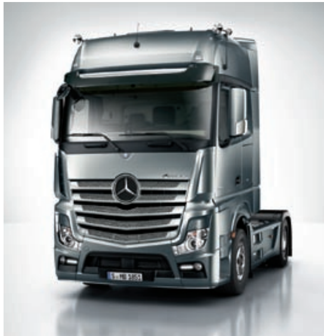
The GigaSpace cab with a width of 2500 mm, a level floor throughout and headroom 1) of 2.13 m, is the largest and most comfortable cab for the new Actros and meets the requirements of international long-distance transport in every respect.
