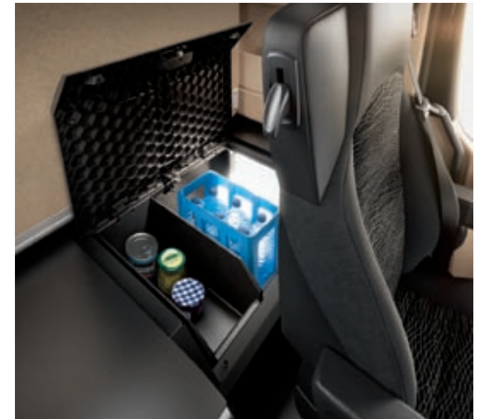
With a stowage capacity of up to 420 l the two stowage compartments under the bed offer plenty of room even for bulky items. They are accessible from both the inside and outside. As an option two sliding and removable stowage trays can be included for smaller items of equipment so that better use can be made of the space available.
