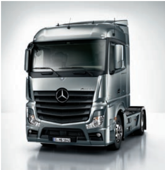
The StreamSpace cab with a width of 2500 mm combines the particularly fuel-saving aerodynamics with an outstanding amount of room and stowage space – ensuring the optimum blend of comfort and economy for applications in international long-distance transport.
