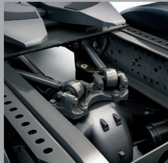
Innovative rear axle guide 1) : instead of a conventional wishbone, two longitudinal control arms whose operating lines' point of intersection is behind the drive axle are used in the new Actros. This results in better directionality, tangibly better understeer/oversteer characteristics and more transverse stability. More about this on pages 38/39.
