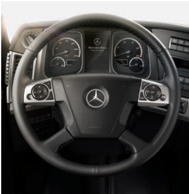
Intuitive operation, easier to climb in and out – with its enlarged adjustment range and eight control buttons on both the right and left, the new standard-specification multifunction steering wheel offers outstanding working comfort. As an option it is also available in leather or a wood/leather combination.
