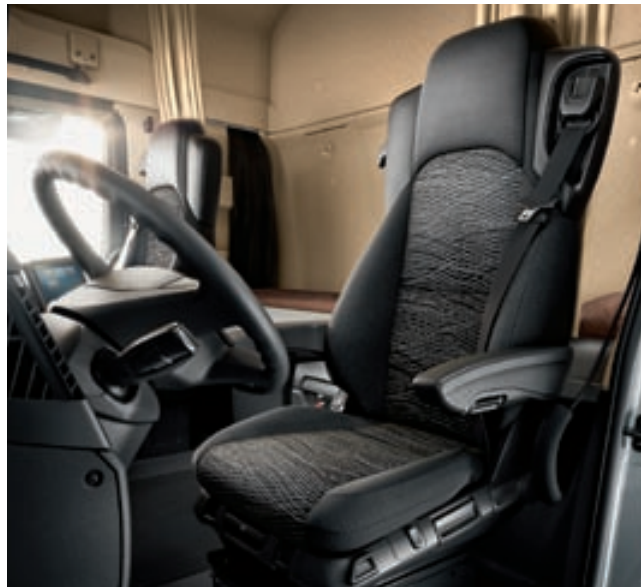
The new comfort suspension seat, with its multiple individual adjustment options, provides excellent seating comfort thanks to features such as the new shoulder adjustment function and the optimised seat cushion inclination adjustment.
